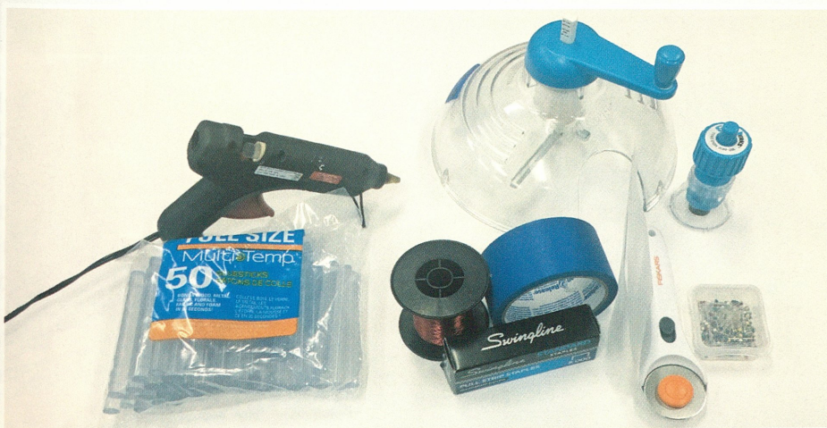
Figure 1: Bioassay cage materials needed include a hot glue gun, glue sticks, circle cutters, tape, monofilament line, stick pins and staples.
