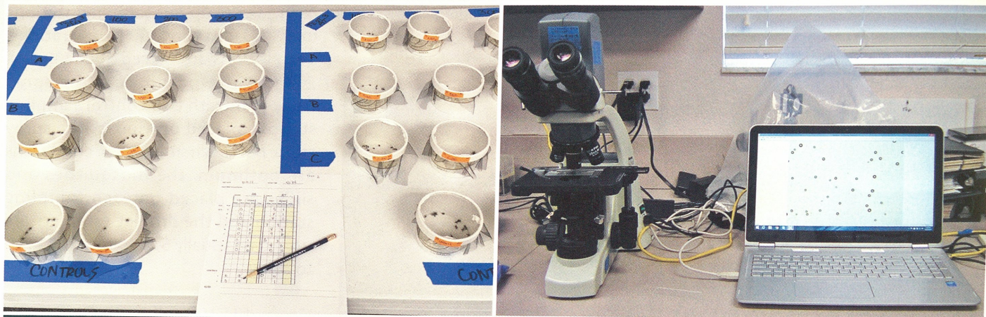
Figure 12: Transfer cups with mosquitoes. Figure 13: Droplet analysis using a compound microscope and DropVision.
